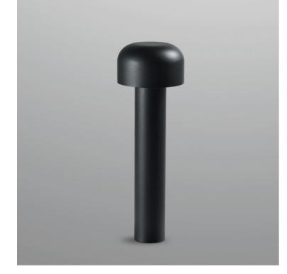
383mm height bollard, for outdoor installation. 360° light emission. Matt black anti-corrosion and UV-proof powder coating. Polycarbonate diffuser, and stainless steel screws. Anchorage bolts included. Built-in LED driver AC100-277V 50/60Hz, power range 7W.
