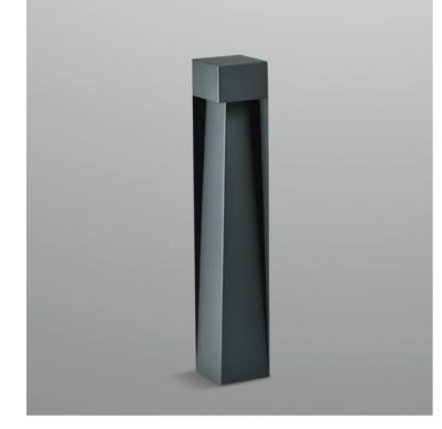
700mm height bollard, for outdoor installation. Dark grey anti-corrosion and UV-proof powder coating. Polycarbonate diffuser, and stainless steel screws. Anchorage bolts included. Built-in LED driver 100-277V 50/60Hz. Wattage Range 6W.
