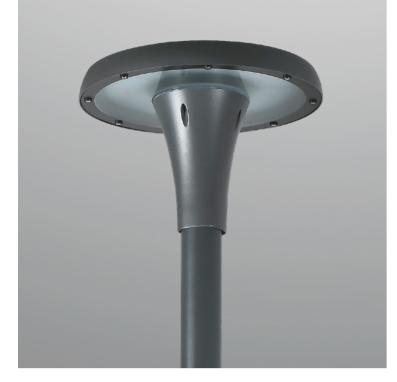
3217mm height, for outdoor installation. 360° light emission. Dark grey anti-corrosion and UV-proof powder coating. Tempered glass diffuser, and stainless steel screws. LED module light source, built-in LED driver AC100-277V 50/60Hz, power range 40-75W.
