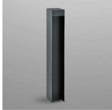
600mm height bollard, for outdoor installation.Dark grey anti-corrosion and UV-proof powder coating. Glass diffuser, and stainless steel screws. Anchorage bolts included. Built-in LED driver 100-277V 50/60Hz. Wattage Range 5-7W.
