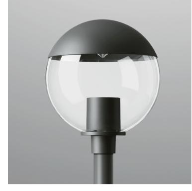
3500mm height, for outdoor installation. 360° light emission. Matt black anti-corrosion and UV-proof powder coating. PMMA diffuser, and stainless steel screws. LED light source, built-in LED driver AC100-277V 50/60Hz, power range 20-30W.
