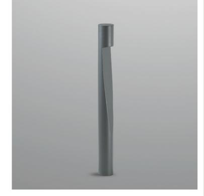
600mm height bollard, for outdoor installation. Dark grey anti-corrosion and UV-proof powder coating. Glass diffuser, and stainless steel screws. Anchorage bolts included. Built-in LED driver 100-277V 50/60Hz. Wattage Range 5W.
