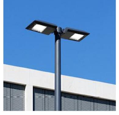
5000mm height, for outdoor installation. 360° light emission. Matt black anti-corrosion and UV-proof powder coating. Stainless steel screws. LED module light source, with 150\*70° beam angle. Built-in LED driver AC100-277V 50/60Hz. Wattage Range 60-120W.
