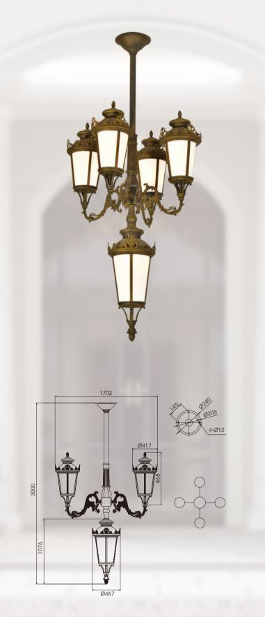
3000mm height, for outdoor installation. 360° light emission. Bronze anti-corrosion and UV-proof powder coating. Polycarbonate diffuser, and stainless steel screws. Suitable for E27 bulb 30-60W, and LED module light source, with 120° beam angle. Built-in LED driver AC100-277V 50/60Hz, power range 30-60W.
