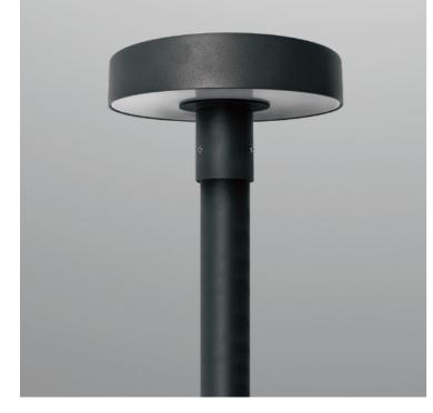
3000mm height, for outdoor installation. 360° light emission. Matt black anti-corrosion and UV-proof powder coating. PMMA diffuser, and stainless steel screws. LED light source, built-in LED driver AC100-277V 50/60Hz, power range 20-50W.
