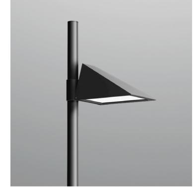
4000mm height, for outdoor installation. 360° light emission. Matt black anti-corrosion and UV-proof powder coating. Stainless steel screws. LED module light source, with 150\*70° beam angle. Built-in LED driver AC100-277V 50/60Hz. Wattage Range 30-60W.
