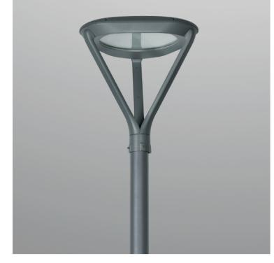
3500mm height, for outdoor installation.  $360^\circ$  light emission. Dark grey anti-corrosion and UV-proof powder coating. Polycarbonate diffuser, and stainless steel screws. LED light source, built-in LED driver AC100-277V 50/60Hz, power range 30-75W.
