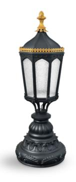
1315mm height, for outdoor installation. 360° light emission. Matt black and golden anti-corrosion and UV-proof powder coating. PMMA diffuser, and stainless steel screws. Suitable for E27 bulb 30-60W, and LED module light source, with 120° beam angle. Built-in LED driver AC100-277V 50/60Hz, power range 30-60W.
