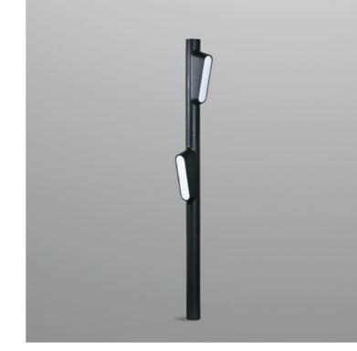
1500mm height bollard, for outdoor installation. Matt black anti-corrosion and UV-proof powder coating. PMMA diffuser, and stainless steel screws. Anchorage bolts included. Built-in LED driver 100-277V 50/60Hz. Wattage Range 2\*12W.
