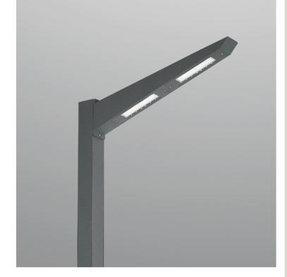
4000mm height, for outdoor installation. Gray metal sand grain anti-corrosion and UV-proof powder coating. Stainless steel screws. LED module light source, with 150\*70° beam angle. Built-in LED driver AC100-277V 50/60Hz. Wattage Range 30-80W.
