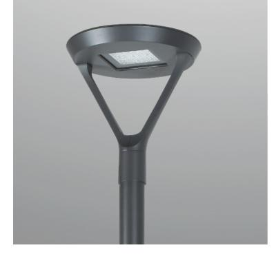
3500mm height, for outdoor installation. 360° light emission. Dark grey anti-corrosion and UV-proof powder coating. Tempered glass diffuser, and stainless steel screws. LED light source, built-in LED driver AC100-277V 50/60Hz, power range 30-75W.
