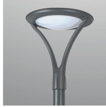
3500mm height, for outdoor installation. 360° light emission. Dark grey anti-corrosion and UV-proof powder coating. Polycarbonate diffuser, and stainless steel screws. LED light source, built-in LED driver AC100-277V 50/60Hz, power range 30-75W.
