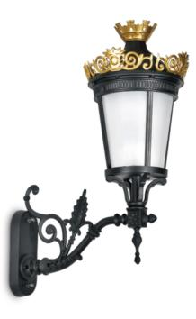
857mm height, for outdoor installation. 360° light emission. Matt black and golden anti-corrosion and UV-proof powder coating. Polycarbonate diffuser, and stainless steel screws. Suitable for E27 bulb 20-35W, and LED module light source, with 120° beam angle. Built-in LED driver AC100-277V 50/60Hz, power range 10-30W.
