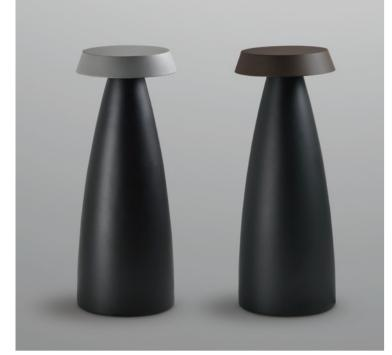
640mm height bollard, for outdoor installation. 360° light emission. Matt black+Matt grey/coffee anti-corrosion and UV-proof powder coating. Polycarbonate diffuser, and stainless steel screws. Anchorage bolts included. Built-in LED driver AC100-277V 50/60Hz, power range 10-20W.
