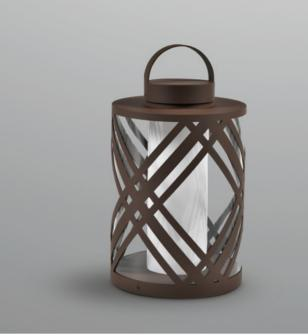
550mm height bollard, for outdoor installation. 360° light emission. Matt coffee anti-corrosion and UV-proof powder coating. PMMA diffuser, and stainless steel screws. Built-in LED driver AC100-277V 50/60Hz, power range 10-20W.
