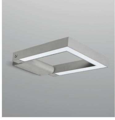
For outdoor installation. Rotatable fixture. Matt grey anti-corrosion and UV-proof powder coating. PMMA diffuser, and stainless steel screws. LED light source, built-in LED driver AC100-277V 50/60Hz, power range 30W.
