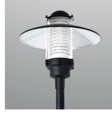
3500mm height, for outdoor installation. 360° light emission. Matt black anti-corrosion and UV-proof powder coating. PMMA diffuser, and stainless steel screws. Suitable for E27 bulb 20-35W, and LED light source, built-in LED driver AC100-277V 50/60Hz, power range 20-40W.
