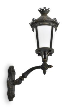
1237mm height, for outdoor installation. 360° light emission. Bronze anti-corrosion and UV-proof powder coating. Polycarbonate diffuser, and stainless steel screws. Suitable for E27 bulb 20-35W, and LED module light source, with 120° beam angle. Built-in LED driver AC100-277V 50/60Hz, power range 20-30W.
