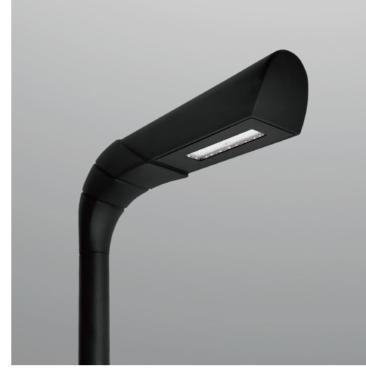
3650mm height, for outdoor installation. Matt black anti-corrosion and UV-proof powder coating. Stainless steel screws. LED module light source, with 150\*70° beam angle. Built-in LED driver AC100-277V 50/60Hz. Wattage Range 30-60W.
