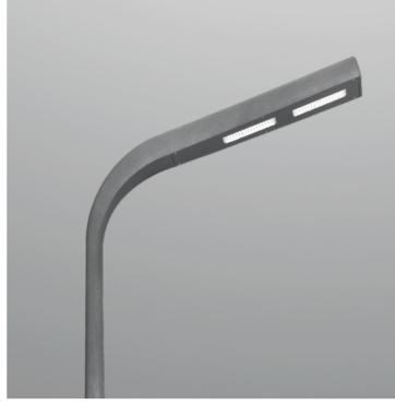
5000mm height, for outdoor installation. Gray Metal sand grain anti-corrosion and UV-proof powder coating. Stainless steel screws. LED module light source, with 150\*70° beam angle. Built-in LED driver AC100-277V 50/60Hz. Wattage Range 30-120W.
