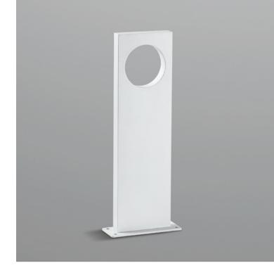
500mm height bollard, for outdoor installation.Matt white anti-corrosion and UV-proof powder coating. Glass diffuser, and stainless steel screws. Anchorage bolts included. Built-in LED driver 100-277V 50/60Hz. Wattage Range 5-7W.
