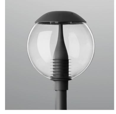
3500mm height, for outdoor installation. 360° light emission. Matt black anti-corrosion and UV-proof powder coating. PMMA diffuser, and stainless steel screws. LED light source, built-in LED driver AC100-277V 50/60Hz, power range 30-40W.
