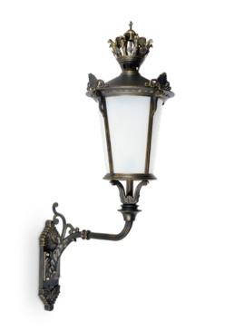
1384mm height, for outdoor installation. 360° light emission. Bronze anti-corrosion and UV-proof powder coating. Polycarbonate diffuser, and stainless steel screws. Suitable for E27 bulb 30-50W, and LED module light source, with 120° beam angle. Built-in LED driver AC100-277V 50/60Hz, power range 30-50W.
