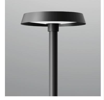
3200mm height, for outdoor installation. 360° light emission. Matt black anti-corrosion and UV-proof powder coating. PMMA diffuser, and stainless steel screws. LED light source, built-in LED driver AC100-277V 50/60Hz, power range 30-50W.
