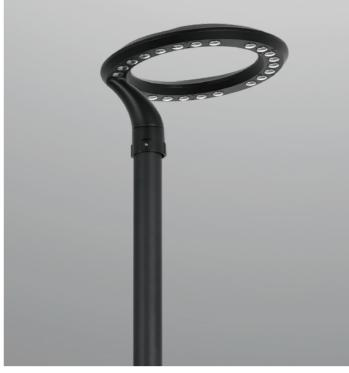
3250mm height, for outdoor installation. 360° light emission. Matt black anti-corrosion and UV-proof powder coating. Polycarbonate diffuser, and stainless steel screws. LED light source, built-in LED driver AC100-277V 50/60Hz, power range 30-50W.
