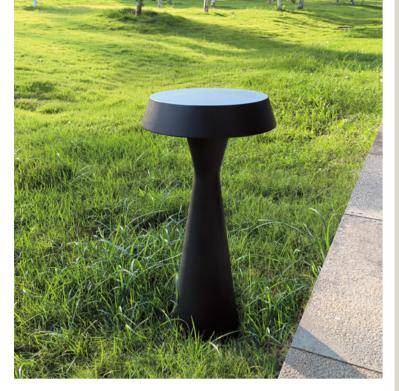
500mm height bollard, for outdoor installation. 360° light emission. Matt black anti-corrosion and UV-proof powder coating. Polycarbonate diffuser, and stainless steel screws. Anchorage bolts included. Built-in LED driver AC100-277V 50/60Hz, power range 10-20W.
