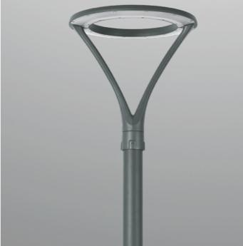
3500mm height, for outdoor installation. 360° light emission. Dark grey anti-corrosion and UV-proof powder coating. Polycarbonate diffuser, and stainless steel screws. LED light source, built-in LED driver AC100-277V 50/60Hz, power range 30-60W.
