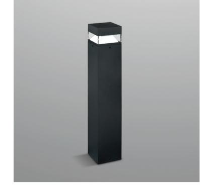
683mm height bollard, for outdoor installation, 360° light emission. Matt black anti-corrosion and UV-proof powder coating. PMMA diffuser, and stainless steel screws. Anchorage bolts included. Built-in LED driver 100-277V 50/60Hz. Wattage Range 10-15W.
