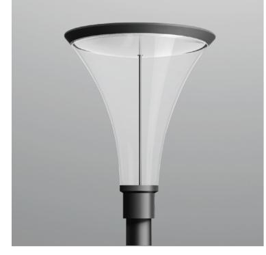
3500mm height, for outdoor installation. 360° light emission. Matt black anti-corrosion and UV-proof powder coating. PMMA diffuser, and stainless steel screws. LED light source, built-in LED driver AC100-277V 50/60Hz, power range 30-50W.
