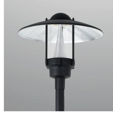
3248mm height, for outdoor installation. 360° light emission. Matt black anti-corrosion and UV-proof powder coating. Stainless steel screws. LED light source, built-in LED driver AC100-277V 50/60Hz. Wattage Range 20-35W.
