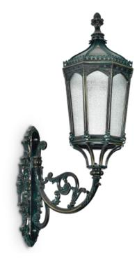
1259mm height, for outdoor installation. 360° light emission. Bronze anti-corrosion and UV-proof powder coating.PMMA diffuser, and stainless steel screws. Suitable for E27 bulb 30-60W, and LED module light source, with 120° beam angle. Built-in LED driver AC100-277V 50/60Hz, power range 30-60W.
