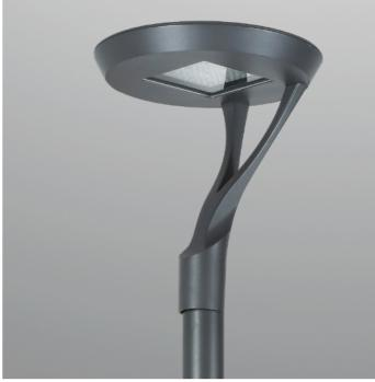
3500mm height, for outdoor installation. 360° light emission. Dark grey anti-corrosion and UV-proof powder coating. Tempered glass diffuser, and stainless steel screws. LED light source, built-in LED driver AC100-277V 50/60Hz, power range 30-75W.
