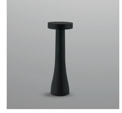
510mm height bollard, for outdoor installation, 360° light emission. Matt black anti-corrosion and UV-proof powder coating. Polycarbonate diffuser, and stainless steel screws. Anchorage bolts included. Built-in LED driver 100-277V 50/60Hz. Wattage Range 7-15W.
