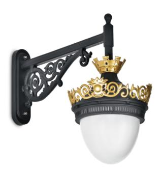
721mm height, for outdoor installation. 360° light emission. Matt black and golden anti-corrosion and UV-proof powder coating. Polycarbonate diffuser, and stainless steel screws. Suitable for E27 bulb 20-35W, and LED module light source, with 120° beam angle. Built-in LED driver AC100-277V 50/60Hz, power range 20-30W.
