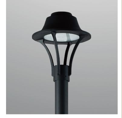
3335mm height, for outdoor installation. 360° light emission. Matt black anti-corrosion and UV-proof powder coating. Tempered glass diffuser, and stainless steel screws. LED light source, built-in LED driver AC100-277V 50/60Hz, power range 20-40W.
