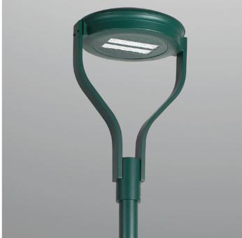
3500mm height, for outdoor installation. 360° light emission. Matt green anti-corrosion and UV-proof powder coating. Stainless steel screws. LED module light source, with 150\*70° beam angle. Built-in LED driver AC100-277V 50/60Hz. Wattage Range 40-120W.
