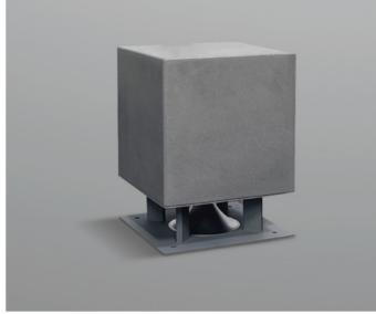
290mm height bollard, for outdoor installation. 360° light emission. Matt grey anti-corrosion and UV-proof powder coating. PC diffuser, and stainless steel screws. Anchorage bolts included. Built-in LED driver AC100-277V 50/60Hz, power range 10-20W.
