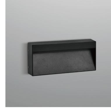
For outdoor installation. Matt black anti-corrosion and UV-proof powder coating. Polycarbonate diffuser, and stainless steel screws. Built-in LED driver AC220-240V 50/60Hz. Wattage Range 5.8W.
