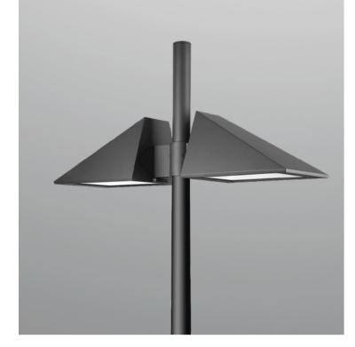
6000mm height, for outdoor installation. 360° light emission. Matt black anti-corrosion and UV-proof powder coating. Stainless steel screws. LED module light source, with 150\*70° beam angle. Built-in LED driver AC100-277V 50/60Hz. Wattage Range 60-120W.
