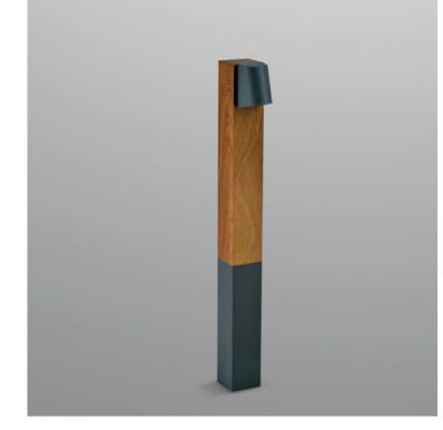
1000mm height bollard, for outdoor installation. Dark grey+wooden grain anti-corrosion and UV-proof powder coating. Glass diffuser, and stainless steel screws. Anchorage bolts included. Built-in LED driver 100-277V 50/60Hz. Wattage Range 5-10W.
