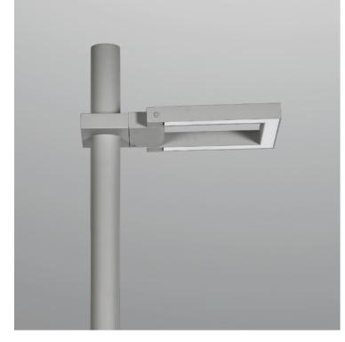
3000mm height, for outdoor installation. Rotatable fixture. Matt grey anti-corrosion and UV-proof powder coating. PMMA diffuser, and stainless steel screws. LED light source, built-in LED driver AC100-277V 50/60Hz, power range 30W.
