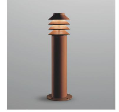
1000mm height bollard, for outdoor installation.Matt red anti-corrosion and UV-proof powder coating. PMMA diffuser, and stainless steel screws. Anchorage bolts included. Built-in LED driver 100-277V 50/60Hz. Wattage Range 10-15W.
