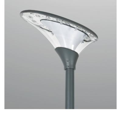
3500mm height, for outdoor installation. 360° light emission. Dark grey anti-corrosion and UV-proof powder coating. Polycarbonate diffuser, and stainless steel screws. LED light source, built-in LED driver AC100-277V 50/60Hz, power range 30-60W.
