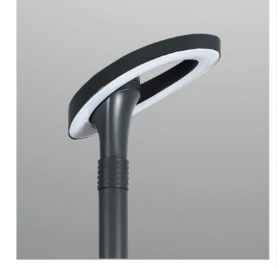
3419mm height, for outdoor installation. 360° light emission. Dark grey anti-corrosion and UV-proof powder coating. PC diffuser, and stainless steel screws. Built-in LED driver AC100-277V 50/60Hz, power range 20-30W.
