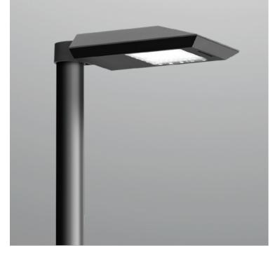
3500mm height, for outdoor installation. 360° light emission. Matt black anti-corrosion and UV-proof powder coating. Stainless steel screws. LED module light source, with 150\*70° beam angle. Built-in LED driver AC100-277V 50/60Hz. Wattage Range 30-60W.
